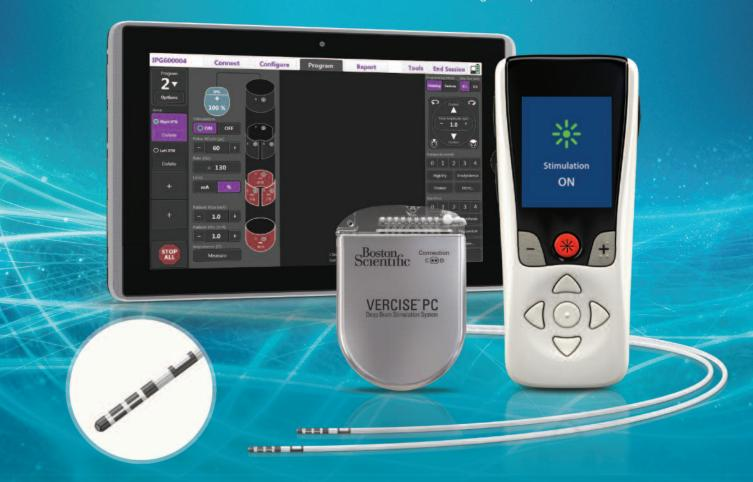
\*Multiple Independent Current Control: 16 independent current sources engineered for fine adjustment of stimulation position and shape
